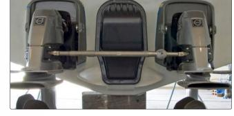
This stern thruster option can also be the best choice for boats without stern drives, if the inside configuration of the boat's stern makes a standard thruster installation impractical.
