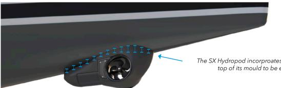
The SX Hydropod incorproates an easy adaptable surface at the top of its mould to be easyily adapted to the hulls shape during installation
